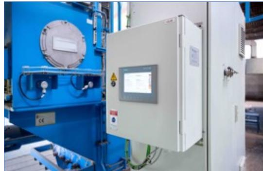
Fig. 1) ALM mounted on the control box of a baling press
