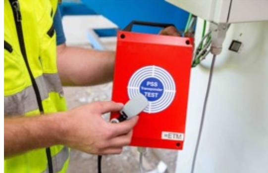
Fig. 4) Test of a P-TAG transponder on the ETM module
