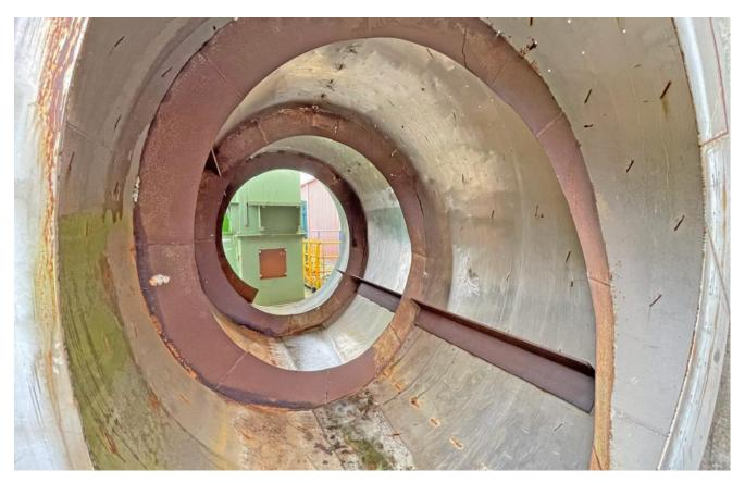
This is a 6000 x 3000 mm bale loosening drum for breaking up and loosening materials pressed into bales.
