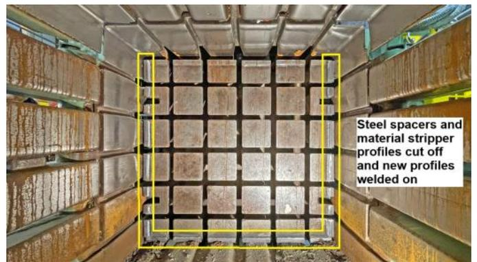
Steel spacers and material stripper profiles cut off and new profiles welded on
