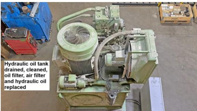
Hydraulic oil tank drained, cleaned, oil filter, air filter and hydraulic oil replaced
