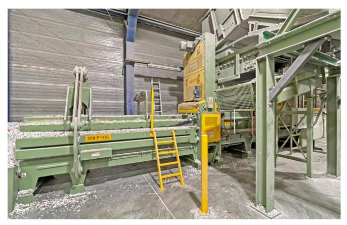
Unlike the standard HBC press series from Bollegraaf, this machine does not have a pre-press flap but cuts the material between blades on the press ram and the counter blade in the frame. This makes it a cutting edge press, similar to a Paal, unoTech, etc. The press is in very good condition for its age, as it was used exclusively for compressing paper from document destruction.
