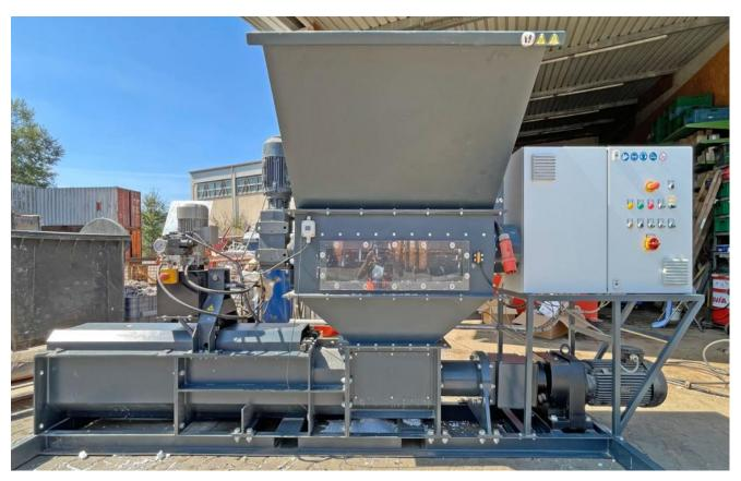
The press was only used sporadically, is in very good condition and available at short notice. Due to the low weight of the machine and the forklift shoes in the transport frame, the press is mobile and can be used directly on the construction site where the material is produced. The electrical connection is made via a CEE 32 A plug.
