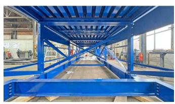
Feed hopper with hydraulic moving floor and bag opener, manufacturer BRT Hartner GmbH, type HP5-3035, yoc 2015, hopper volume 30 m³
