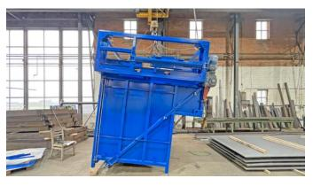
Feed hopper with hydraulic moving floor and bag opener, manufacturer BRT Hartner GmbH, type HP5-3035, yoc 2015, hopper volume  $30\ m^3$
