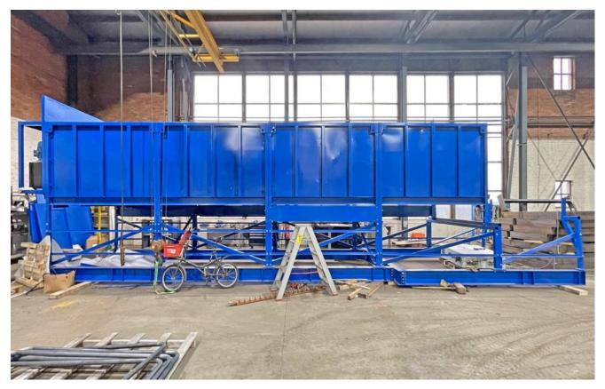
The feed hopper with bag opener was in use at a large recycling company, where waste in bags was tipped into the hopper with wheel loaders and the bags were opened via the bag opener and the waste was conveyed in doses for further processing. The system worked perfectly until it was dismantled and was replaced by a larger system with a higher throughput capacity. The machine is in good working condition.
