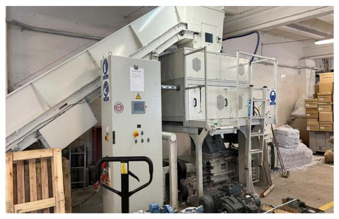
This is a complete system consisting of a feed conveyor belt, a two-stage shredder and a horizontal baling pres.
