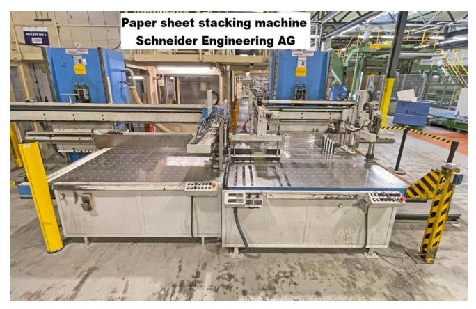
It is a destacking and restacking machine for paper and cardboard.
