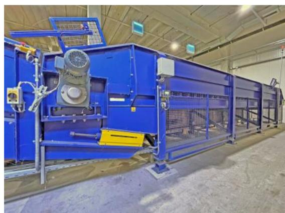
**Bale opener and bale dewiring system, yoc 2015, only approx. 3,500 operating hours, throughput approx. 50 bales per hour, with weighing system**
