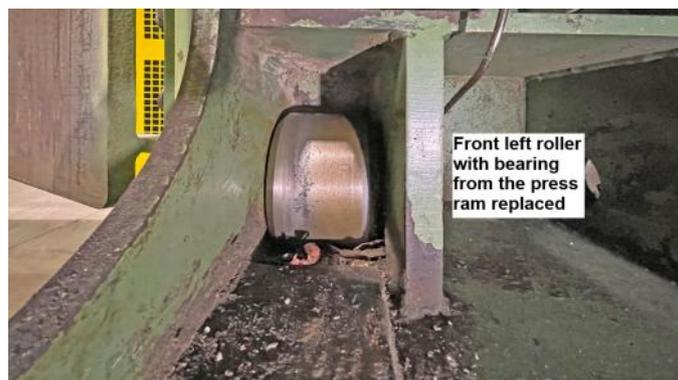
Front left roller with bearing from the press ram replaced
