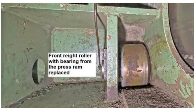
Front right roller with bearing from the press ram replaced
