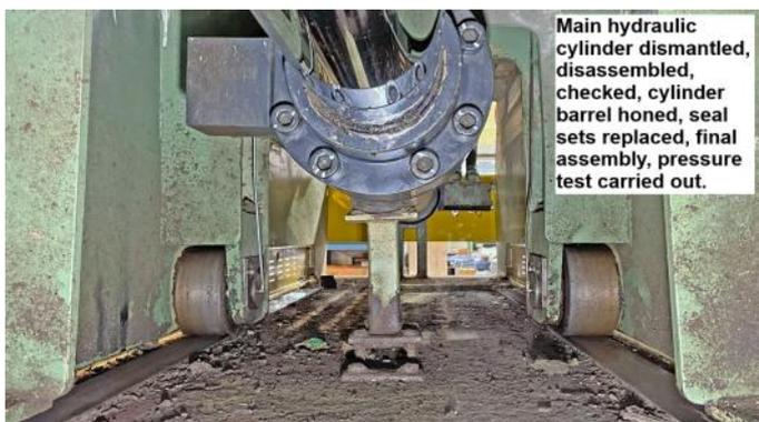
Main hydraulic cylinder dismantled, disassembled, checked, cylinder barrel honed, seal sets replaced, final assembly, pressure test carried out.
