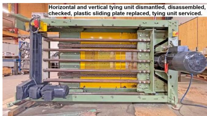
Horizontal and vertical tying unit dismantled, disassembled, checked, plastic sliding plate replaced, tying unit serviced.
