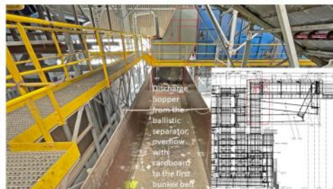
Overflow (cardboard) from the ballistic separator
