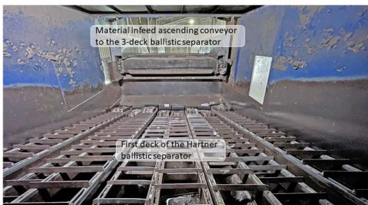
Material infeed ascending conveyor to the 3-deck ballistic separator
