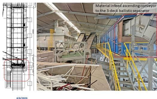
Material infeed ascending conveyor to the 3-deck ballistic separator
